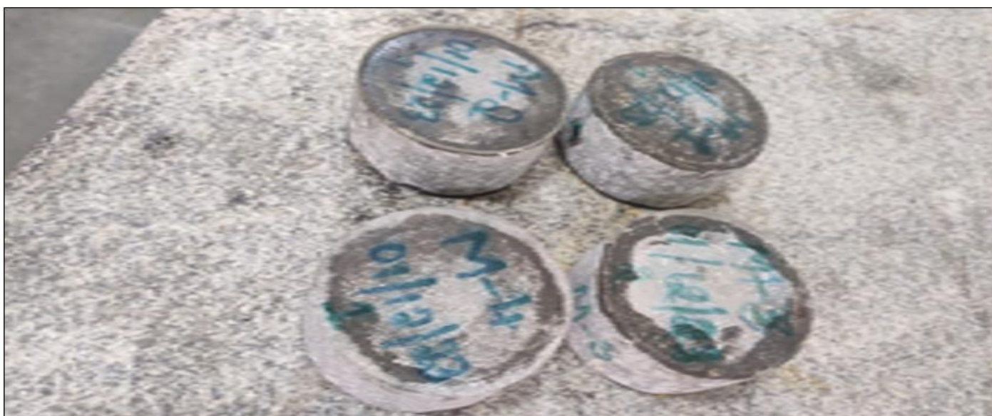
Fig 1 Cut and epoxy coated specimens before testing
