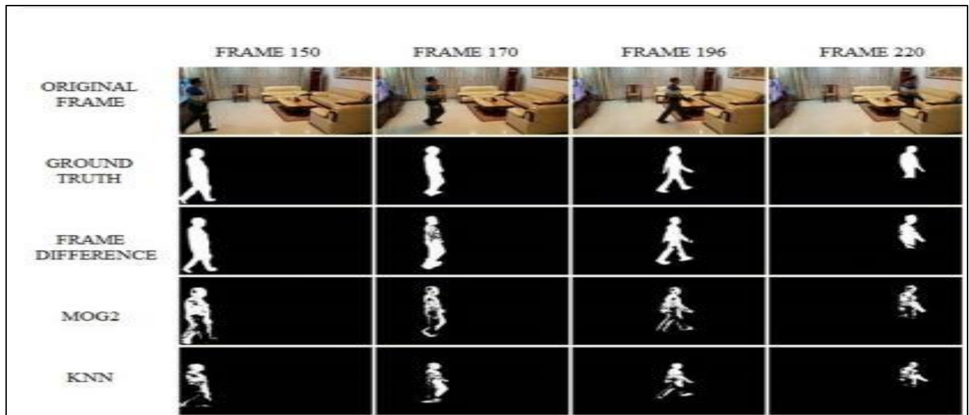
Fig 2: Comparison of Different Background Subtraction Techniques
