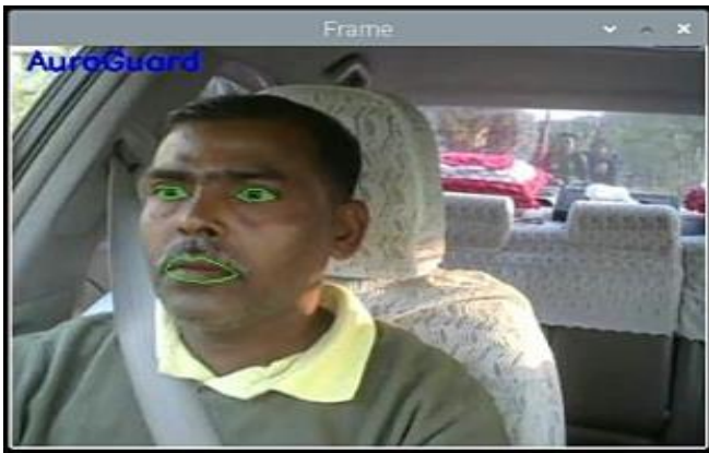
Fig 18 Facial Landmark Detection for Real time Monitoring. The system uses OpenCV's facial landmarking algorithms to identify and track key facial points such as eyes, nose, and lips.
