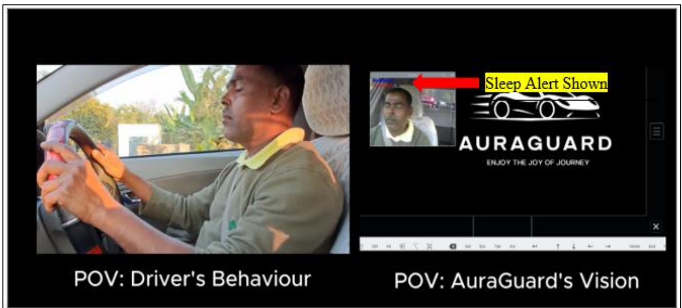
Fig 22 Visualization of the Driver Sleep Alert system in action. The left frame captures the driver's physical behavior showing signs of drowsiness, while the right frame illustrates how AuraGuard: SDS's vision system detects and analyzes the driver's eye closure to trigger a sleep alert for early intervention.
