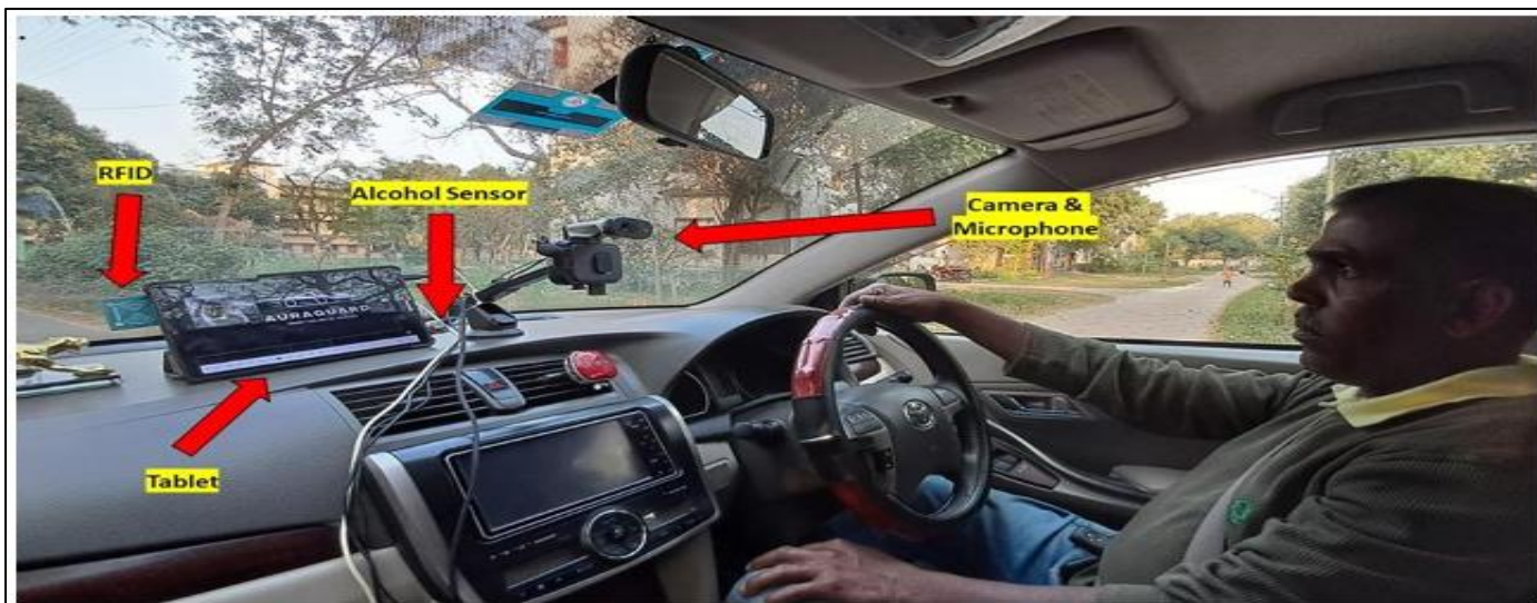
Fig 16 System Setup into a real car
