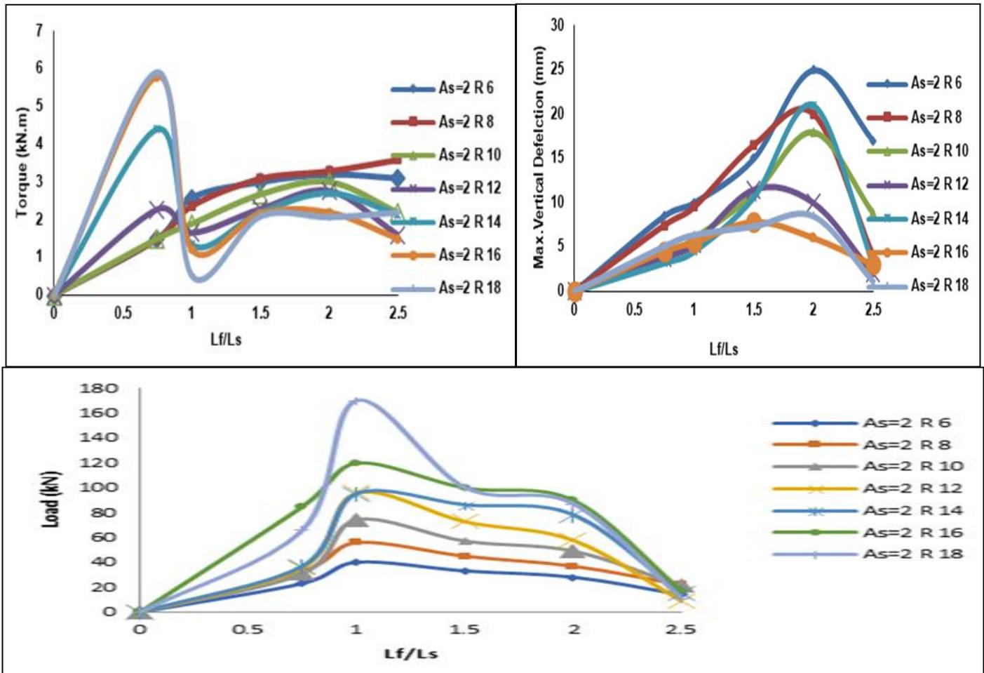
Fig 4: Relation between the Ultimate Load, Max. Deflection and Ultimate Torque with  $L_f/L_s$  Ratios for Different Steel Reinforcement of the Floor Beams
