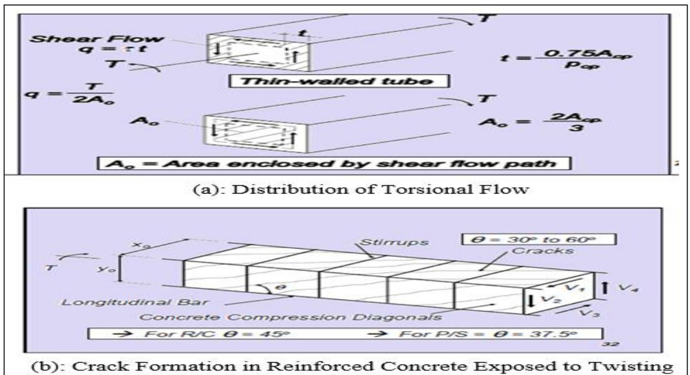
Fig 2: Space Truss Analogy: (a): Distribution of Torsional Flow, (b) Cracks Generation.<sup>[3]</sup>
