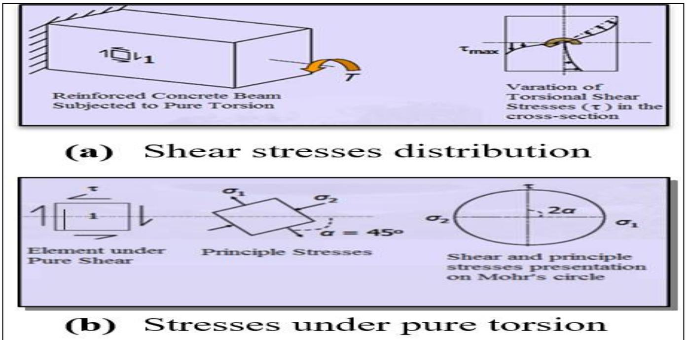
Fig 1: Reinforced Concrete Element Subjected to Pure Torsion
