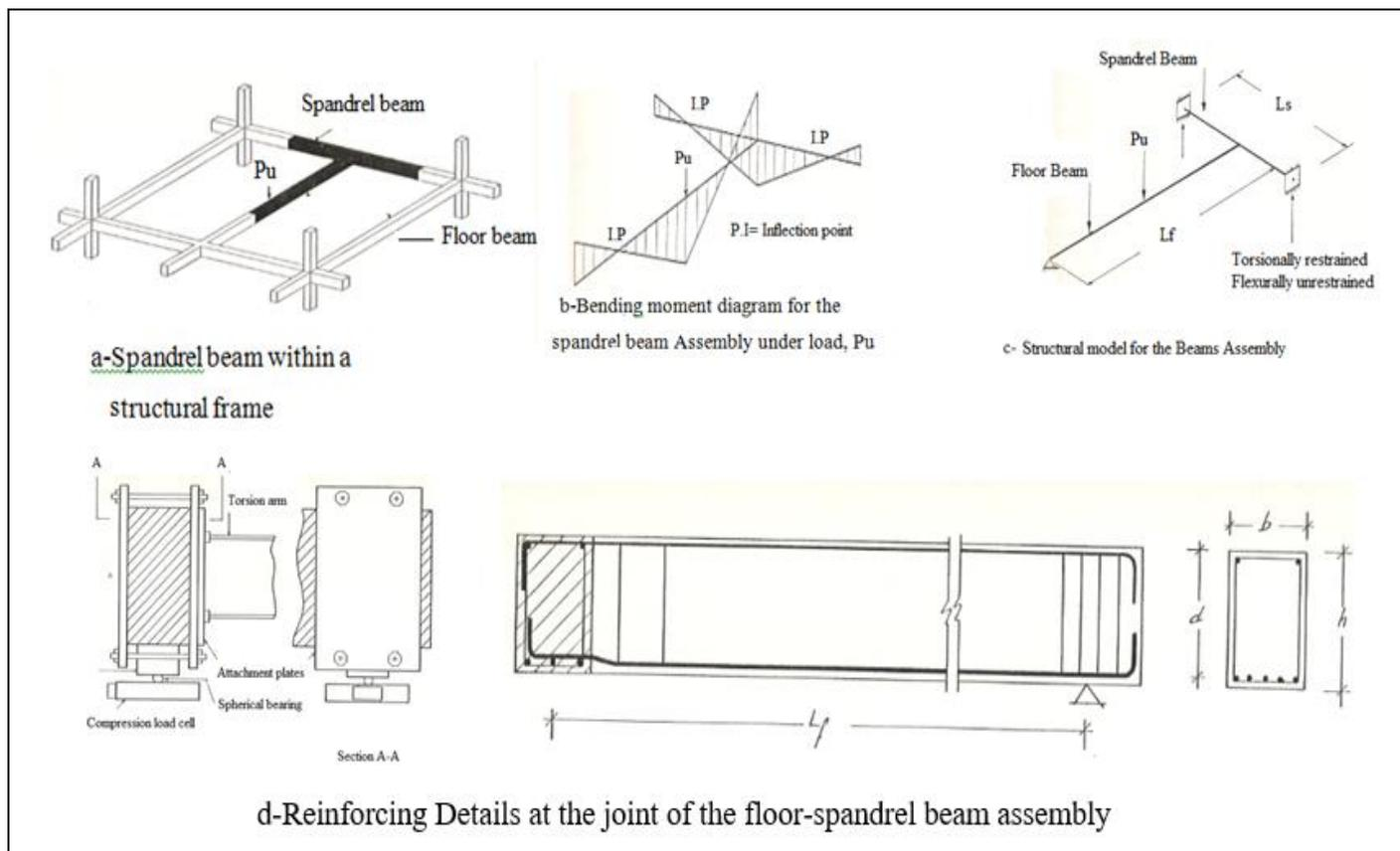
Fig 3: Typical Details for the Tested Spandrel-Floor Beams Assembly [11].
