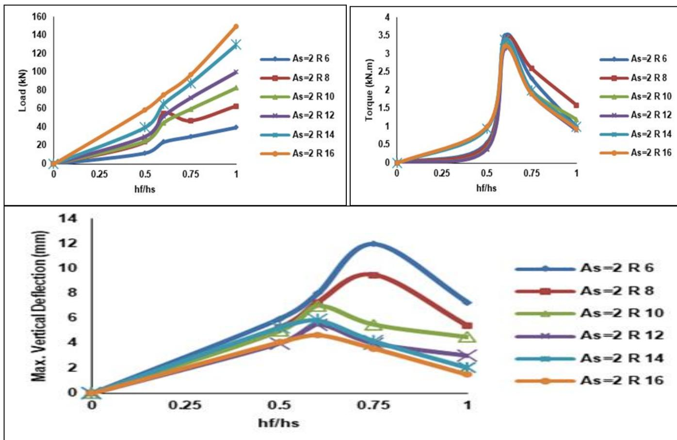
Fig 5: Reinforcement Effects on the Analysis Results for Different  $h_f/h_s$  Ratios
