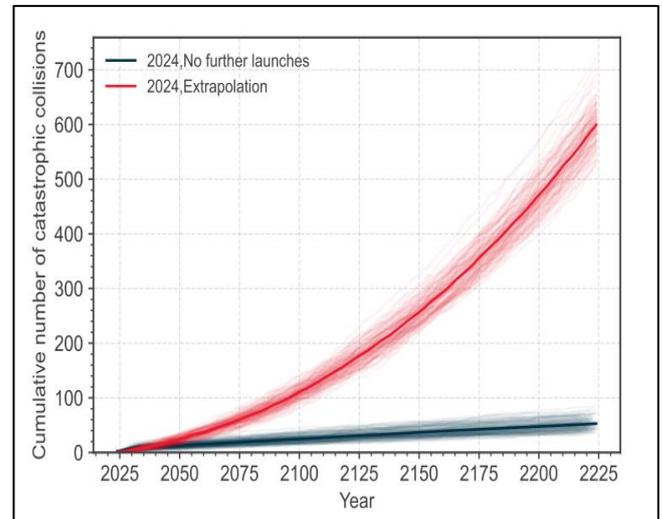
Fig 6: Simulated Long-Term Evolution Scenarios Depicting Cumulative Collisions in LEO
