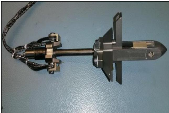
Fig 8: The Harpoon Mechanism on the Remove Debris Satellite is Engineered to Spear and Pull in Floating Debris from Earth's Orbit. [Image Source: Airbus/the RemoveDebris Consortium] [67]
