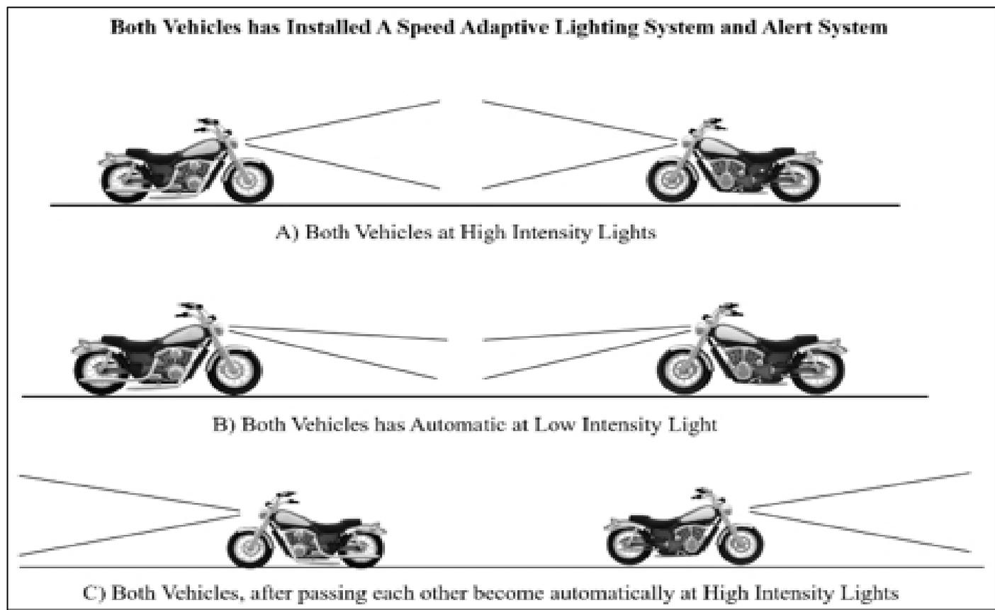
Fig 2: Detection of a Approaching Vehicle Headlight
