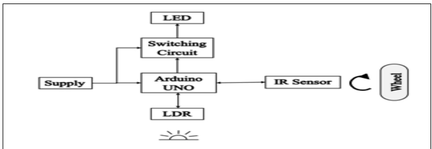
Fig 1: Basic Block Diagram of Working System
