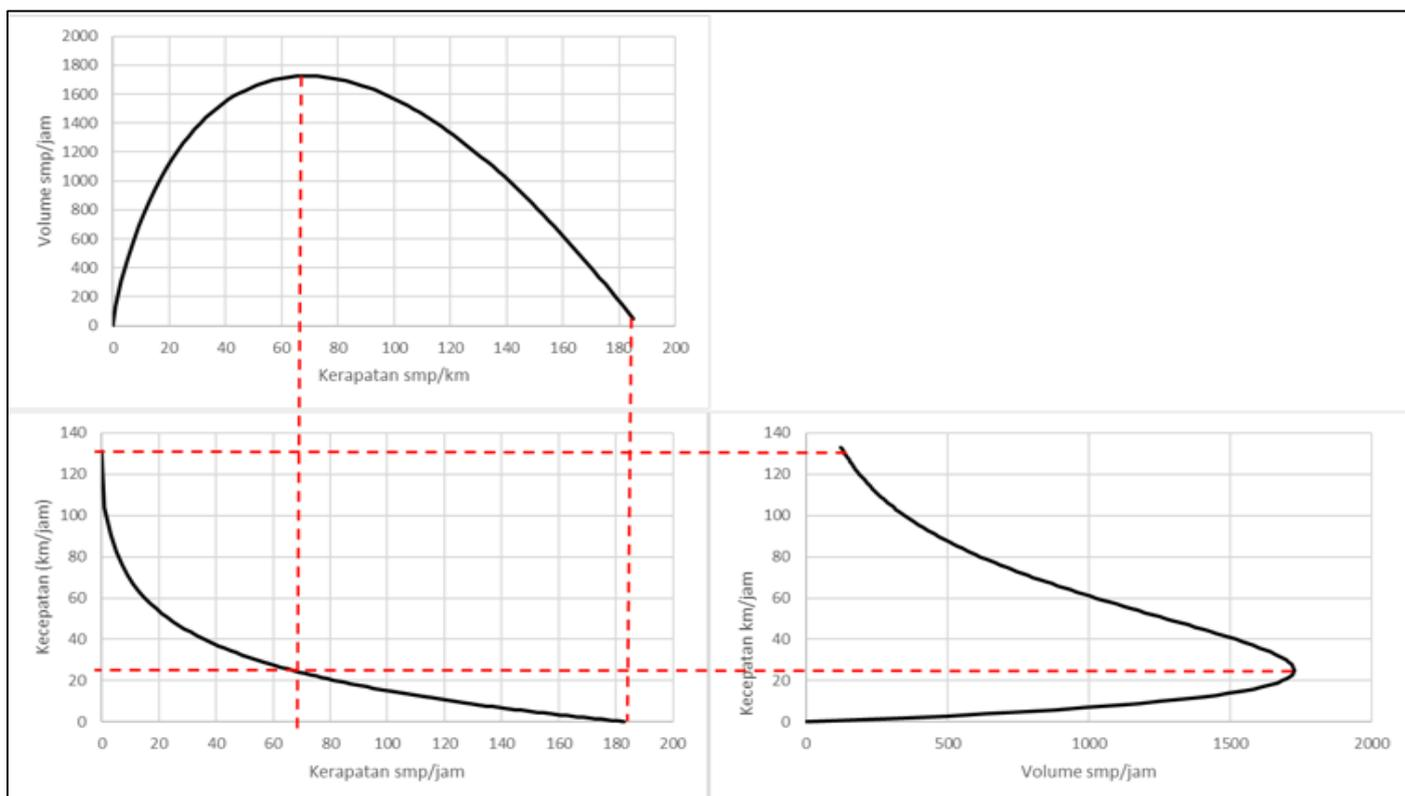
Fig 9: Graph of the Relationship Between Volume, Velocity, and Density of the Greenberg Model
