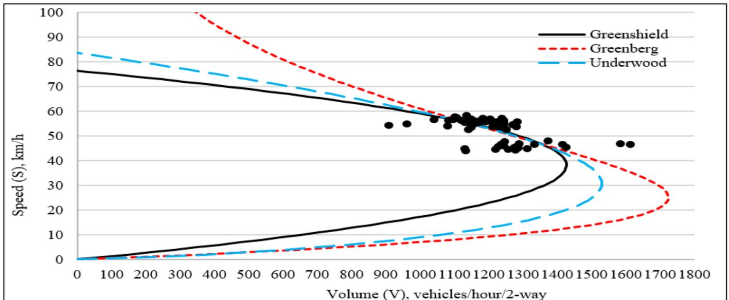
Fig 5: The Relationship between S-V Conditions and Heavy Vehicles (HV)
