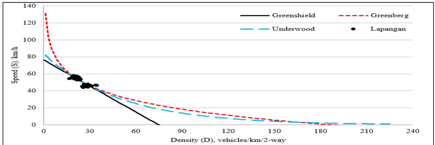
Fig 3: The Relationship between S-D Conditions and Heavy Vehicles (HV)
