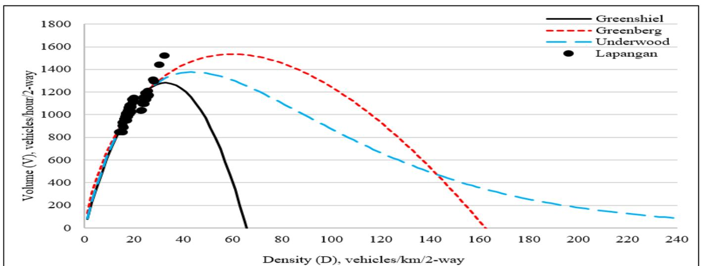
Fig 7: V-D Relationship in a Scenario without Heavy Vehicles (HV)
