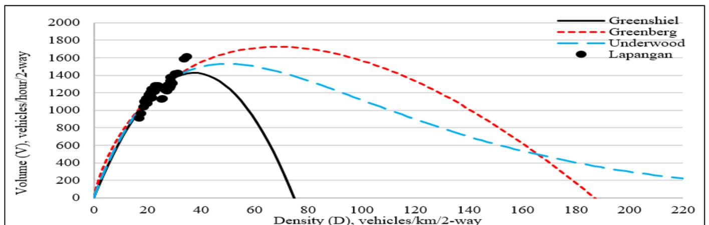
Fig 4: The Relationship between V-D Condition and Heavy Vehicles (HV)
