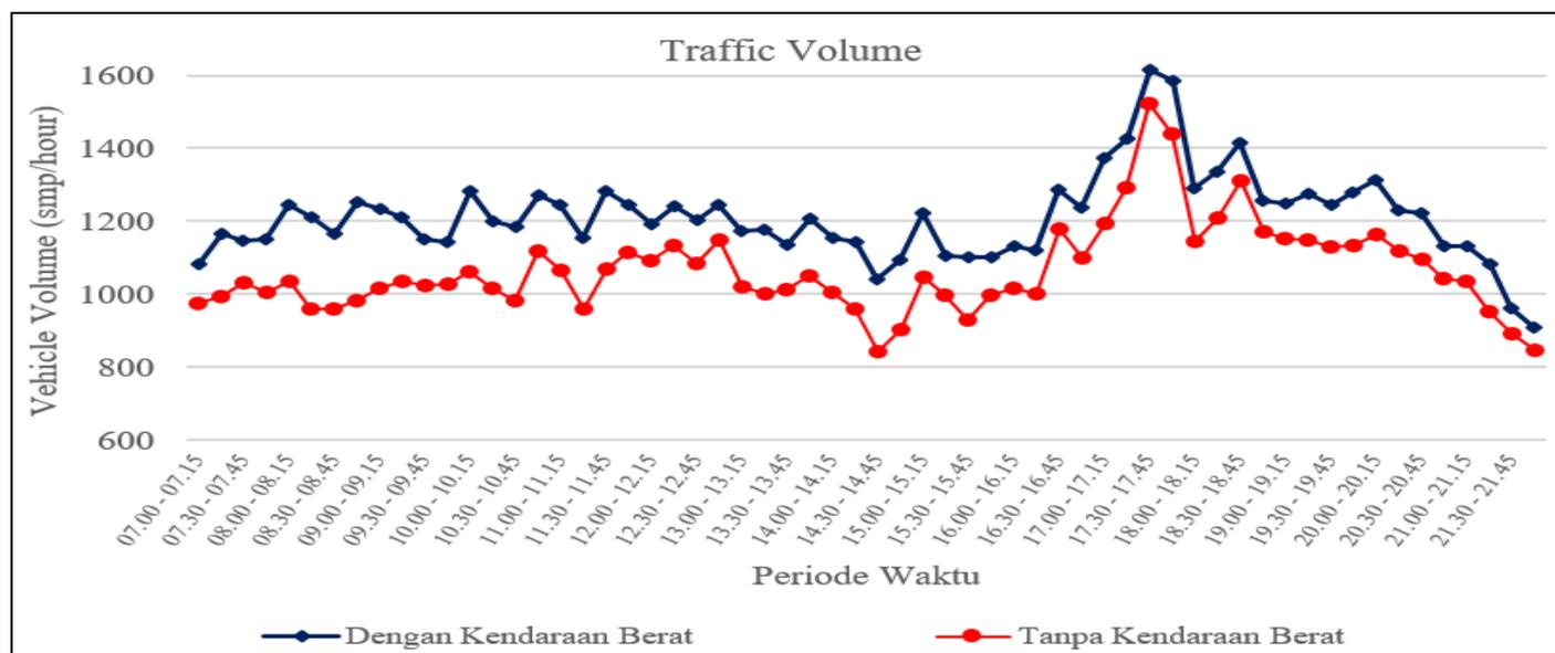
Fig 2: Peak Traffic Volume Graph (Each Condition)
