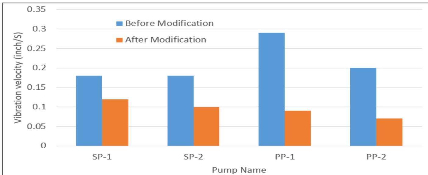
Fig 7 Peak Velocity (inch/sec) of Vibration before and after the Modification
