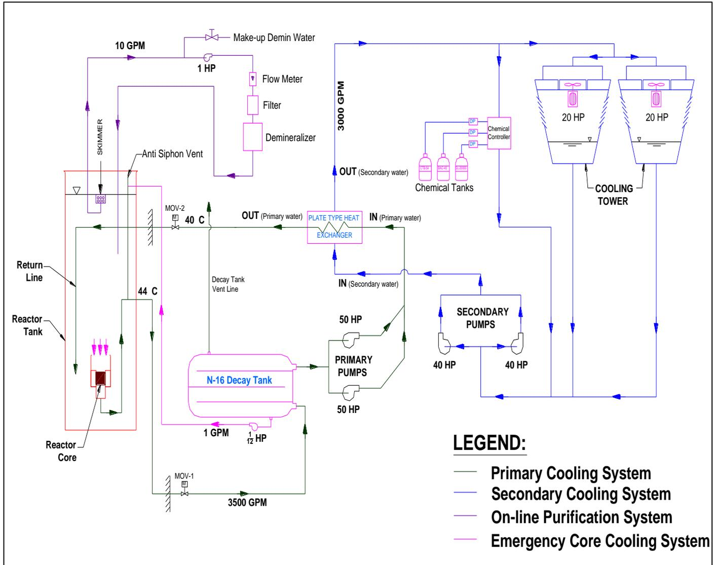
Fig 1 BTRR colling system schematic diagram.
