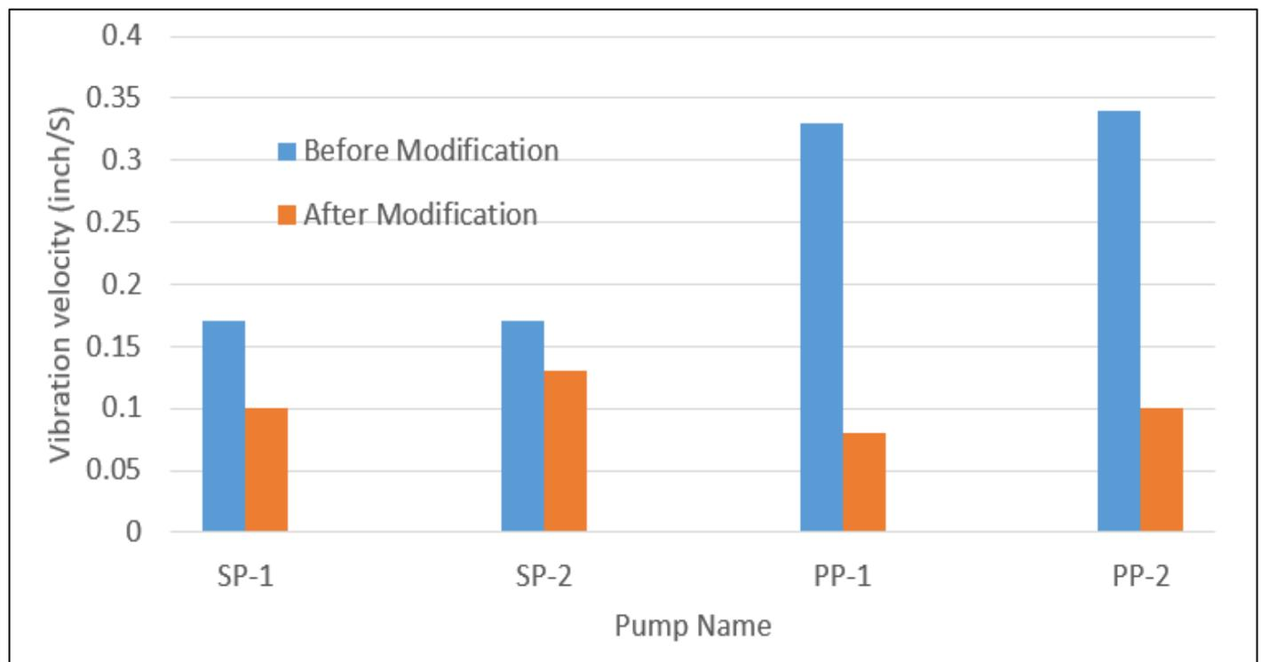
Fig 9 Peak Velocity (inch/sec) of Vibration before and after the Modification
