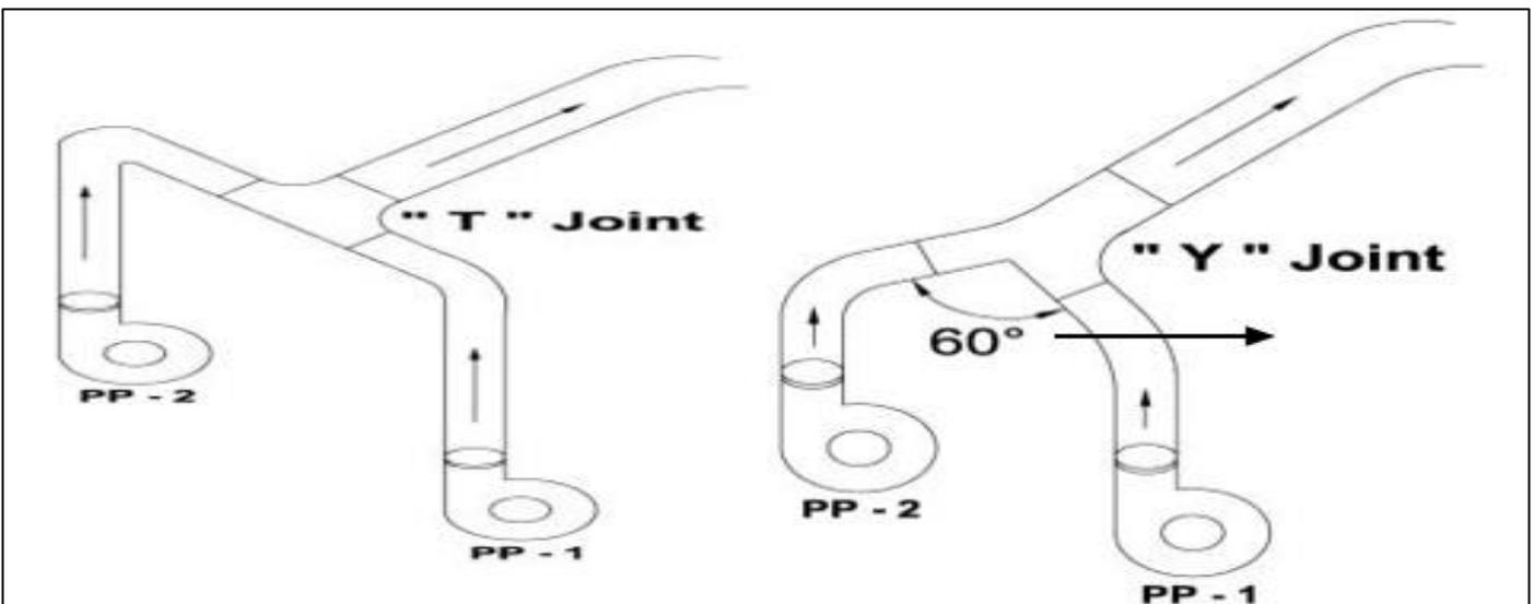
Fig 12 Transformation of Piping Arrangement to Reduce Vibration
