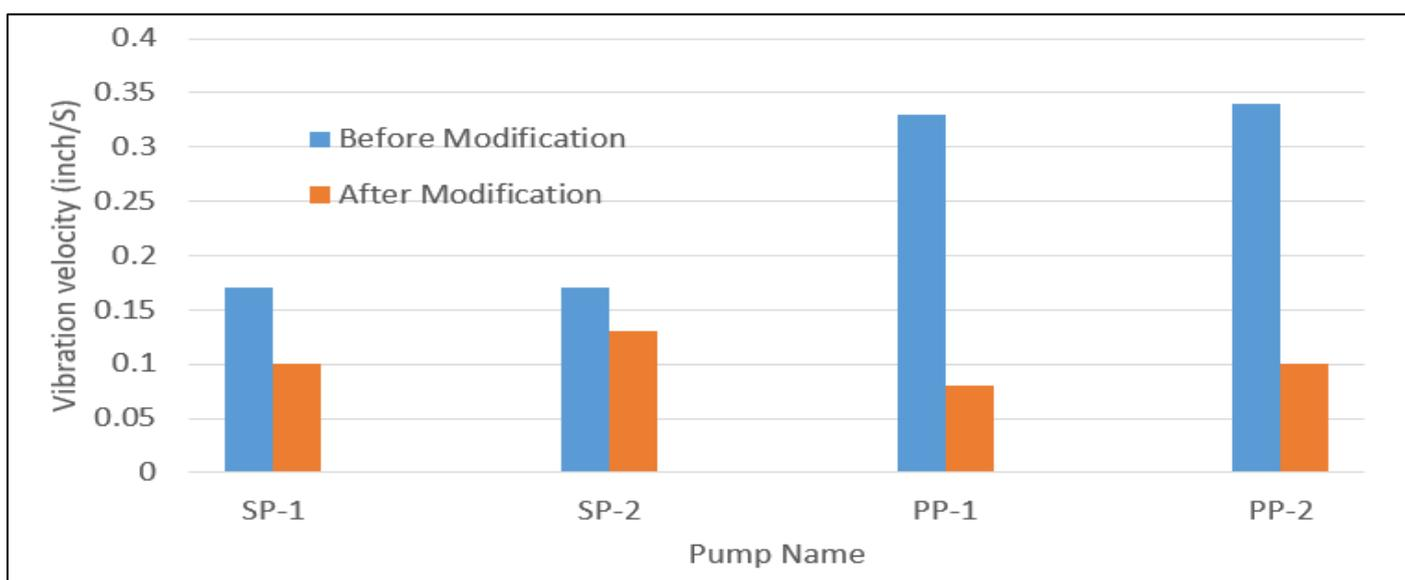
Fig 8 Peak Velocity (inch/sec) of Vibration before and after the Modification
