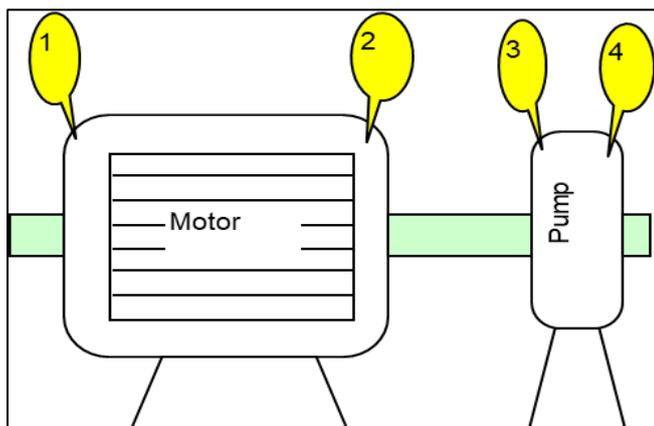
Fig 5 Schematic Diagram of Vibration Measurement Positions.
