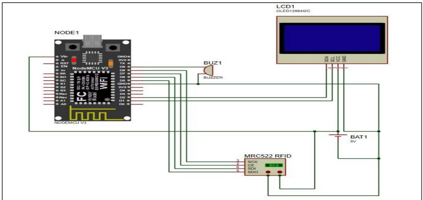
Fig 4 System Circuit Diagram
