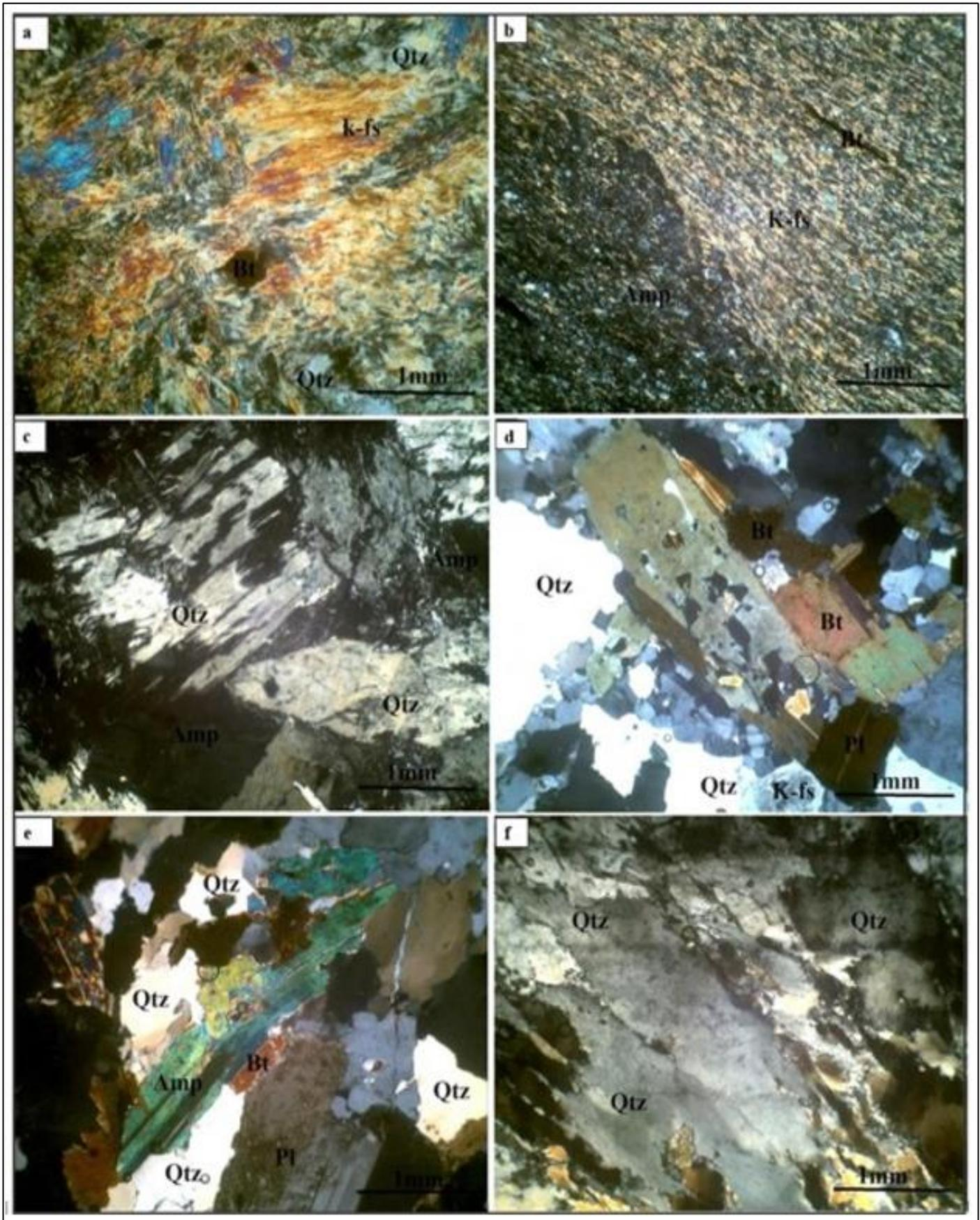
Fig 4 (a,b) Photomicrograph of schist showing quartz (Qtz), K-feldspar (K-fs), amphibole (Amp) and Biotite (Bt); c photomicrograph of amphibolite showing Quartz (Qtz) and amphibole (Amp) ; (d,e) Photomicrograph of granitoids showing quartz (Qtz), biotite (Bt), plagioclase (Pl), K-feldspar (K-fs); and amphibole (Amp) ; (f) Photomicrograph of quartz vein showing quartz (Qtz).
