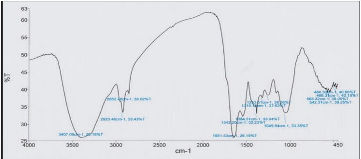
Fig 2: FTIR Spectrum of Ag-NiNPs
