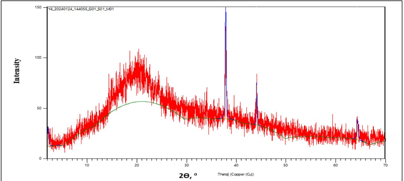
Fig 4: XRD Patterns of Ag-Ni NPs
